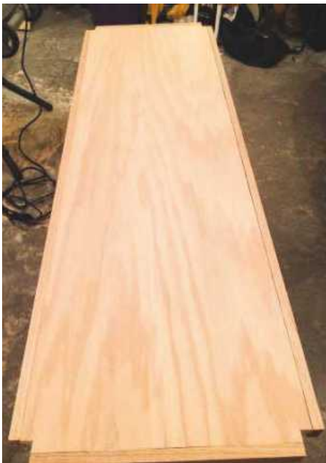
STEP 3. Glue and finish, then nail edge pieces to the top and bottom
